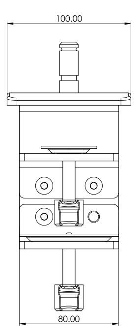
BOTTOM CLAMP CAN BE FITTED TO FOUR DIFFERENT POSITION TO COVER THE FULL RANGE OF DESK THICKNESS. (01-07-2022)
